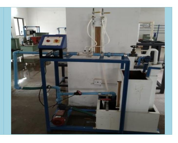
**11.** Orifice meter setup.
